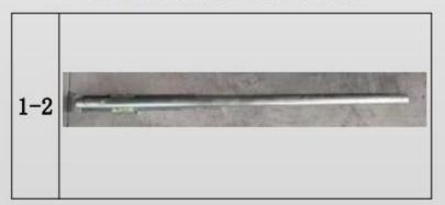
put it in feature for checking the hole location.
